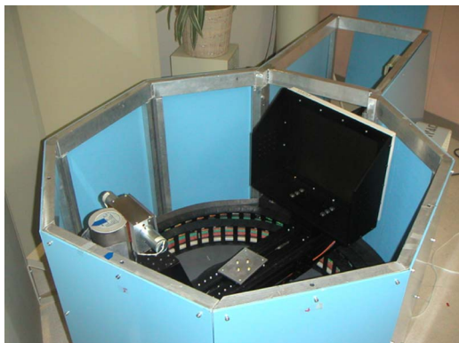
FIG. 1. The first prototype breast CT scanner at our institution, code-named Albion , is pictured. The water-cooled tungsten anode x-ray tube is seen in the foreground, and the flat panel detector system is positioned at the other end of the gantry arm. The system is shown with the patient tabletop removed.
